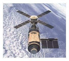
Weighing 75 Metric tons, Skylab was launched 14 May 1973 by a Saturn INT-21 (a two-stage version of the Saturn V launch vehicle) into a 235 nautical mile (435 km) orbit. The launch is sometimes referred to as Skylab 1, or SL-1. Severe damage was sustained during launch, including the loss of the station's micrometeoroid shield/sun shade and one of its main solar panels. Debris from the lost micrometeoroid shield further complicated matters by pinning the remaining solar panel to the
