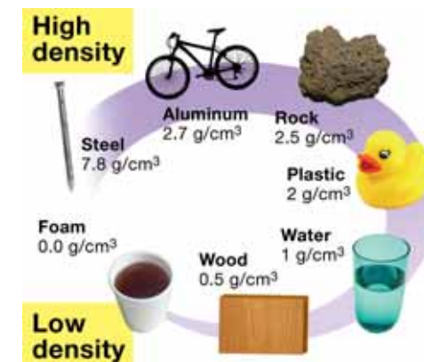
Figure 4.3: The density range of common materials.
